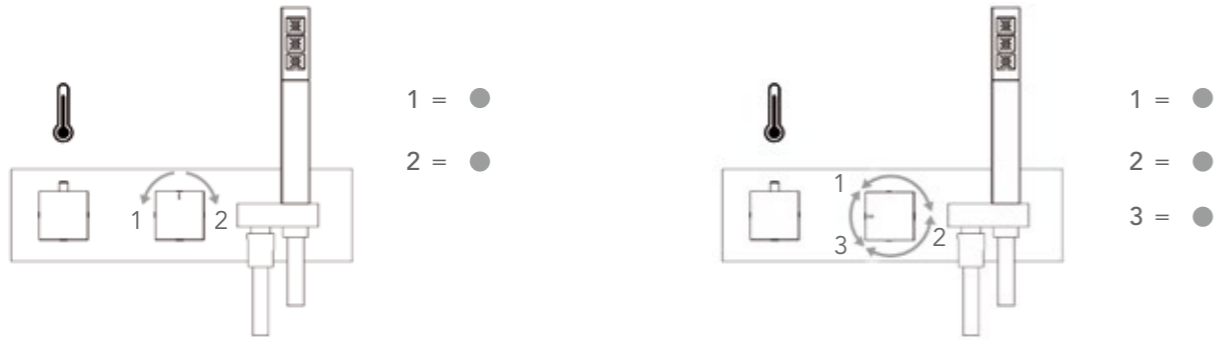
4-WAY, 5-WAY OR 6-WAY MIXER (opening up to 2 outlets simultaneously)
